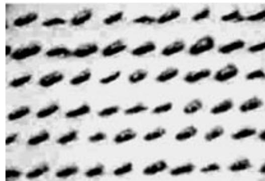
**Fig. 4.** Image of the recrystallized material found on the surface of Fe:LiNbO<sub>3</sub> when the laser is focused in the air ( $3 \mu\text{m}$  above the sample) as viewed from the direction of excitation.
