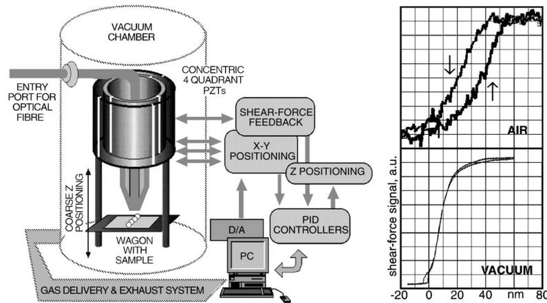
Fig. 1. Left: schematic of the vacuum shear force microscope. Right: typical shear force approach (arrow down) and retreat (arrow up) curves. These curves are taken under ambient and vacuum conditions (after 50' at 2.7 Pa).
