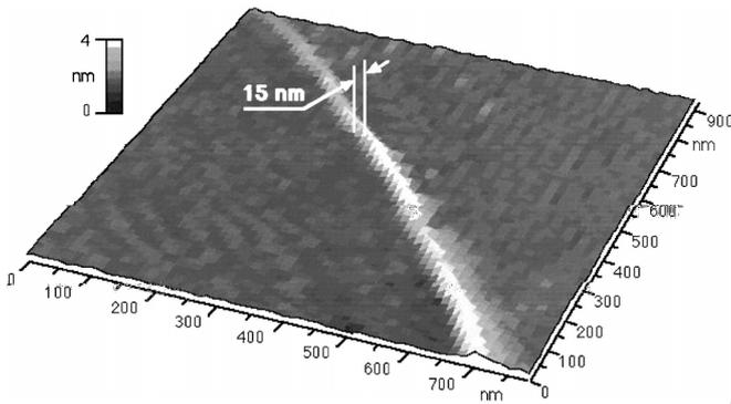
Fig. 3. VSM image of Zinc lines written on Corning glass substrate by means of NFO-PCVD. The vacuum shear force mechanism is used not only to image the Zinc deposit but also to maintain a constant separation between the substrate and the NFO probe during patterning. The probe used in this case had a 100 nm light emitting aperture.
